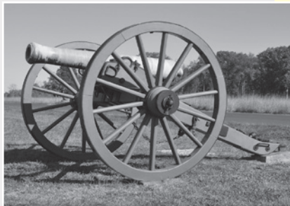
12-pounder Bronze Napoleon, Model 1857 (USA) A muzzle loading gun. The tube was made of Bronze (90% Copper and 10% Tin) and had a muzzle swell. The tube was a smooth bore of 4.62 inches. Fired a 12 pound shell with a range of about 1600 yards. Powder charge was 2.5 pounds. The guns could fire Solid Shot, Spherical Case, Grape and Canister.
