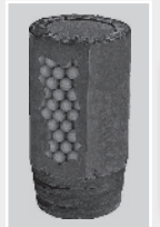
12-pounder Canister Round - about 28 iron round balls inside
