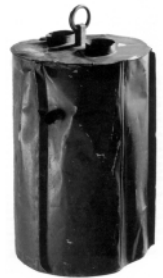
This mine was set off by pulling a lanyard from the shore... later fitted with an electronic detonator connected to the shore by wires... West Point Museum Scanned Photo from Time Life Books
