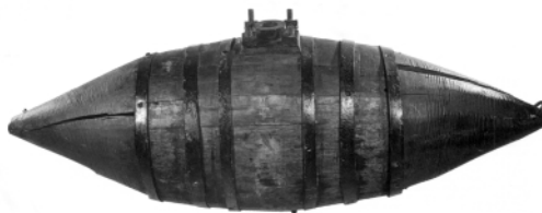
Keg torpedeo, most common, made from beer kegs... West Point Museum Scanned Photo from Time Life Books
